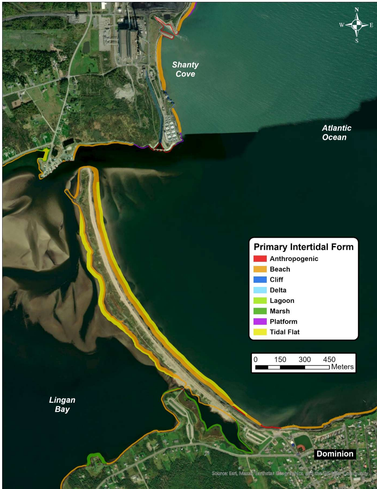
Figure 5. Example of the ShoreZone Primary Intertidal Form displayed as intertidal polygons near Lingan Bay.
